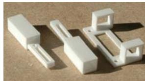
As a by-product of the 3D manufacturing process, some white powder may still be packed inside the tie-bar ends and in the holes. This can be dislodged with a cocktail stick and cleaned up using a 0.90mm – 1.00mm drill twisted by hand in the holes.
