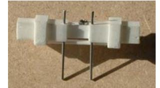
Adjust the distance between the two tubes to roughly match the holes in the baseboard and adjust the tubes so that the top ends will be about 1mm below the baseboard surface when in position.
