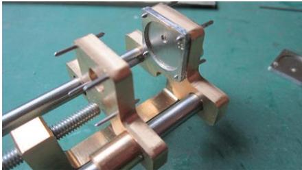
Remove the frame around the etching and fold the etching concertina style. Again, a number 60 drill is useful to run through the holes in the plates. It gives a nice push fit on the pins.
